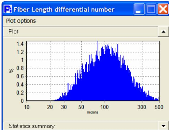
Figure 3: Shows the average length of the fibers to have a mean of 123  $\mu\text{m}$  with a standard deviation of 74.8  $\mu\text{m}$ .
