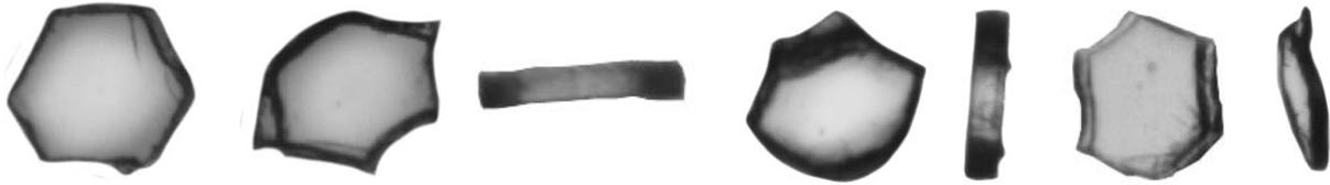
Figure 2. Typical particle thumbnails from a Dynamic Image Analysis system. Notice random orientation allows the analysis of all dimensions of the particle, not just the largest area
