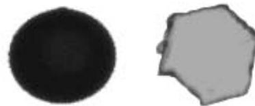
*Figure 1. Although both yield similar results in equivalent spherical diameter, the sphere on the left is actually quite different from the flat disc on the right. A system that orients the largest area of the particle at the viewing point would be unable to see all dimensions of the particle.*
